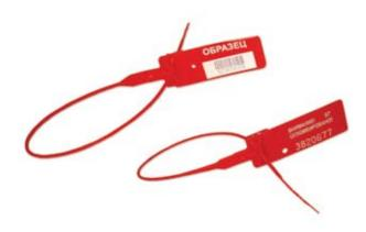
Alfa-M2 seal is an adjustable seal with a round smooth tail, 2 mm diameter. To prevent tampering, this security seal houses the metal insert welded into the locking chamber. There is an additional hole on the seal's flag to fix the spare part of the seal's tail or to apply additional tag. The seals are produced in blocks of ten pieces.
